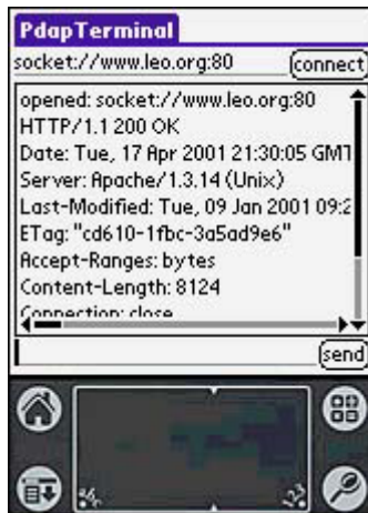
Listing 6.2 MidpTerminal.java—The MIDP Terminal Application for Using Different Protocols in the Same Application
