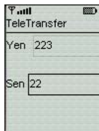
Figure 3.5. The TeleTransfer MIDlet extended to change the labels depending on the state of the currency ChoiceGroup .
